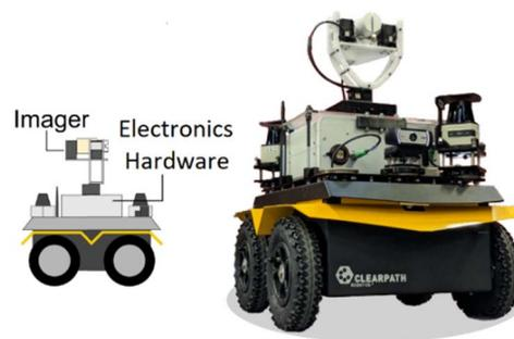
Fig. 1. Integrated radiation detection instrumentation with robotic platform (side elevation, left, front, perspective view, right).
