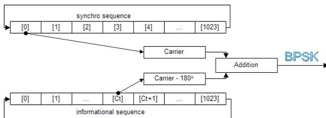
Fig.5– Modulation scheme
